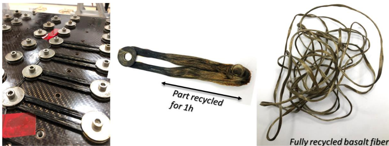
Figure 1. Left. GRAM winding of basalt fiber impregnated with a vitrimer. Middle. Half-recycled composite parts. Right. Fully recovered basalt fiber after chemical degradation of the vitrimer.
